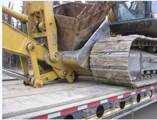
No means of securement on hoe travelling down road
