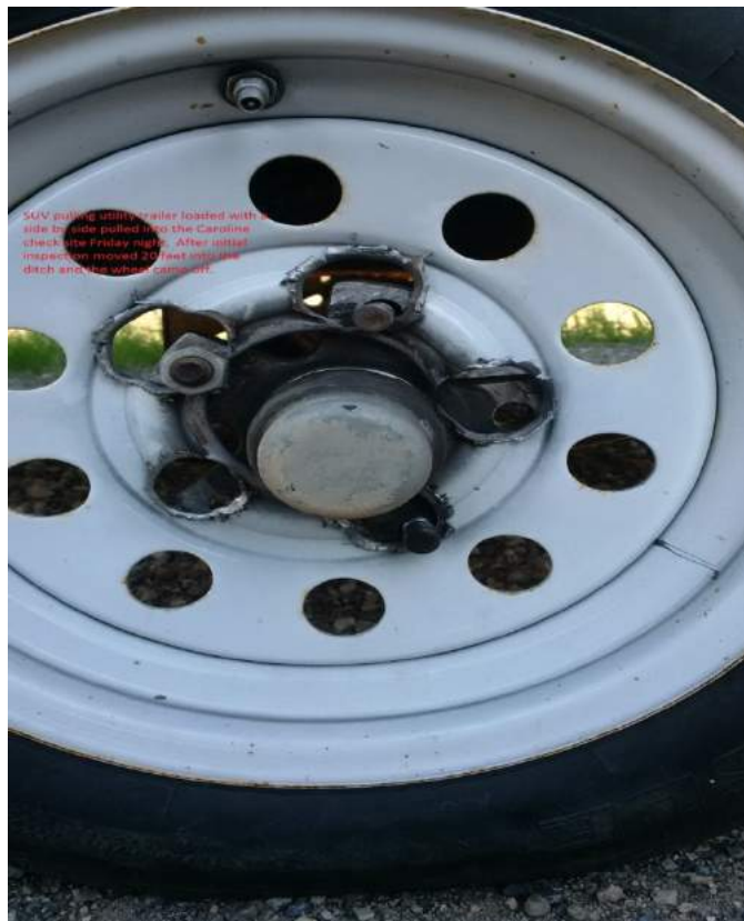
Photos provided by CVE – Trailer hitch not latched (top photo) and an SUV pulling utility trailer loaded with a side-by-side came into Caroline check stop. After initial inspection, asked to pull 20 feet into the ditch for further inspection and wheel came off (bottom photo)
