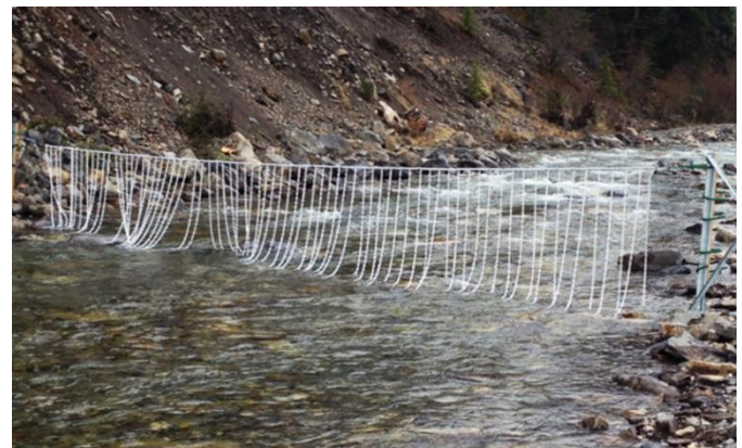
Figure 5: Fence design for watercourses: plastic chain curtain on Panther River test fence in BNP.
